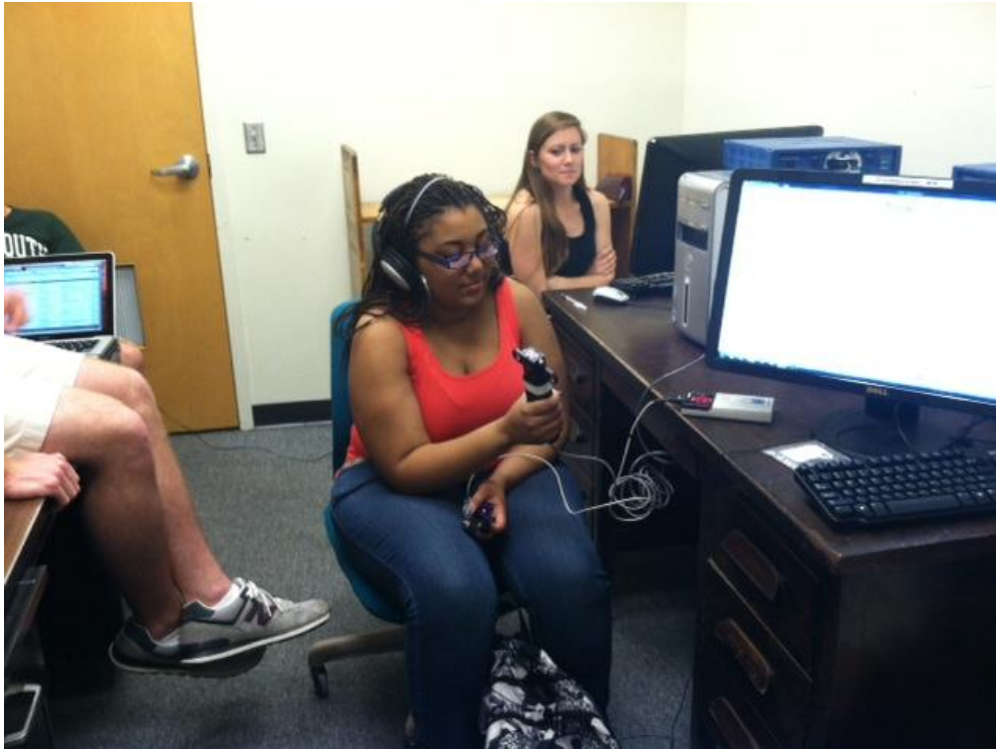
Figure 8. The subject is currently holding the hand dynamometer after listening to the rock audio clip. The BIOPAC system on the far computer is measuring the force of each of these clenches. The BIOPAC system on the near computer is measuring electrodermal activity which is attached to her index and middle fingers.
