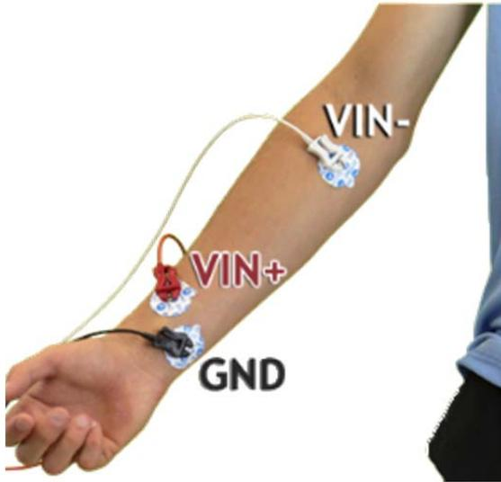
**Figure 2:** The configuration in which the three electrodes from the EMG were attached to each subject's arm (source: Biopac manual).
