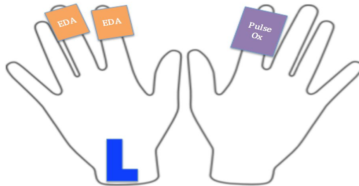
Figure 4. Electrodermal activity (EDA) sensing skin conductance finger electrodes were placed on the participant's left index and middle fingers. The pulse oximeter was clipped on participant's right index finger.
