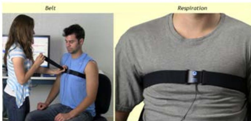
**Figure 1.** Recommended setup for BIOPAC respiratory belt. (Image from BIOPAC tutorial)
