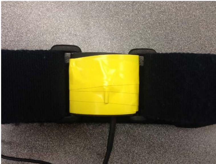
**Figure 7.** Respiration belt repaired with vinyl tape.
